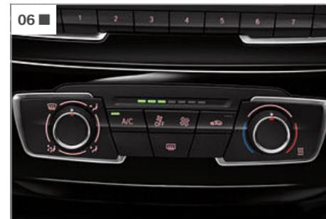
**[ 07 ]** The automatic air conditioning with two-zone control includes Automatic Air Recirculation (AAR) with an active carbon filter, as well as fogging and solar sensors.
